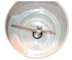
Hold plugs in place for vacuuming
