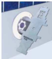
7. Install/remove Hayward jet nozzle retaining ring.
