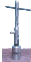
5. Attach tool. Turn clockwise to remove anchor.
