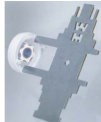
8. Install/remove broken Hayward retaining ring tips.
