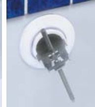
4-5. Install/remove universal wall fittings. Place hex bar in hole for more turning and torque.
